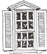
Wood pediment Louvered wood shutters
